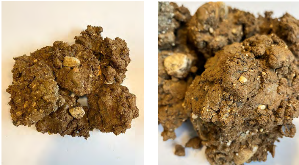
Figure 1. Example of a subsoil suitable for a CobBauge structural layer. Photos: Katey Oven.
