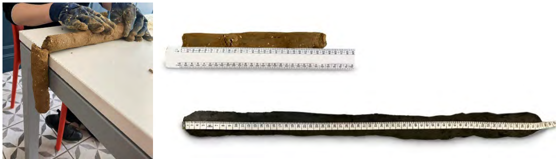
Figure 13 Results for Cigar test methodology, for two different earths, to establish clay type and cohesiveness. Photos: Olivia Elsey.
