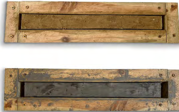
Figure 15 Results for the Shrinkage Box test methodology, for two different earths, to establish clay type and cohesiveness.
