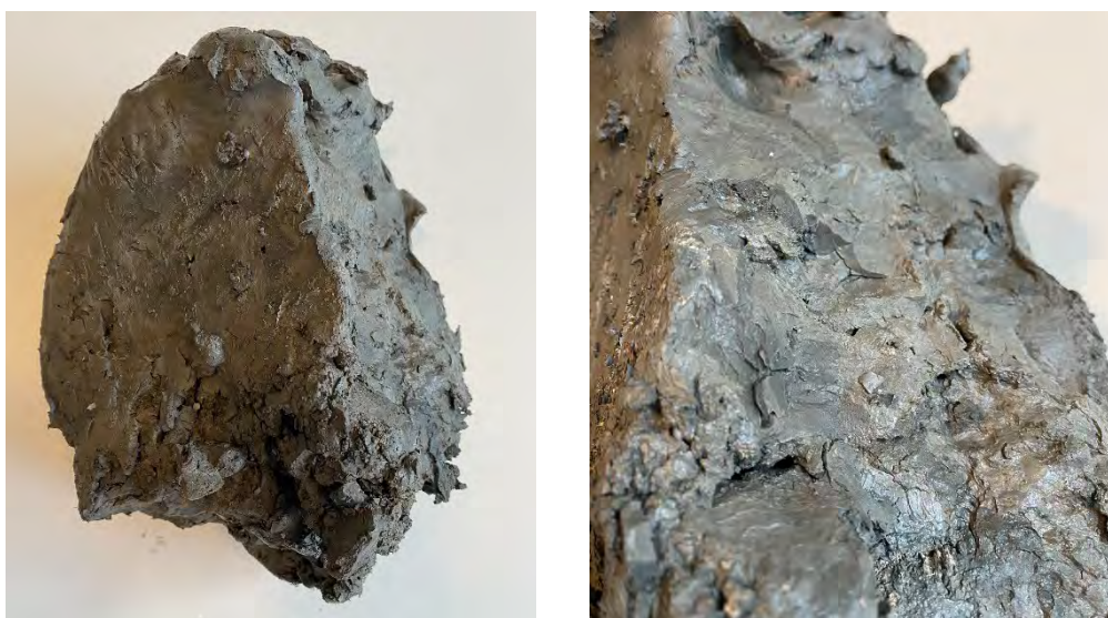
Figure 2. Example of a subsoil suitable for a CobBauge thermal layer. Photos: Katey Oven.
