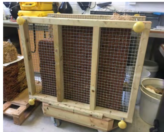
Figure 21. Metal (left) and timber (right) formwork examples. Photos: Esitc Caen (2022) (left), Plymouth University, CobBauge project (2021).
