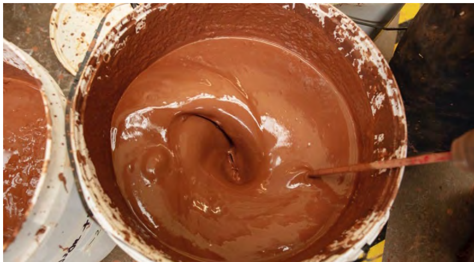
Figure 7. The desired consistency of the clay slip. Photo: François Streiff.
