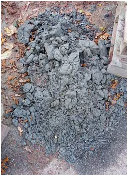
>>> Photo 7. Heaps of clay being weathered before use at a flooring tile factory. The grey clay was sourced from Jurassic Kimmeridge Clay at Setch Road, Middleton, and the purplish clay in the background is pottery clay from Triassic Keuper Marl deposits near Stoke on Trent.
