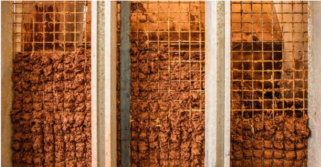
Figure 33. Photo showing the compaction of the light earth viewed through mesh. Photo: Plymouth University, CobBauge project.
