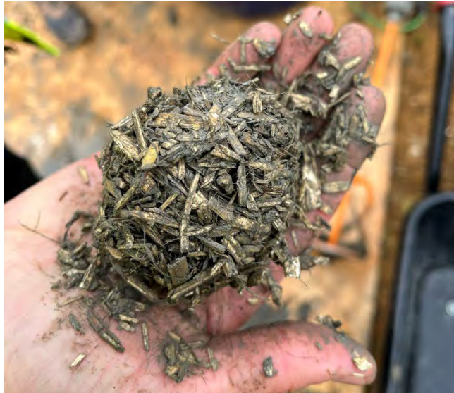
Figure 11. Desired consistency of light earth mix. Photo: Katey Oven (2022).
