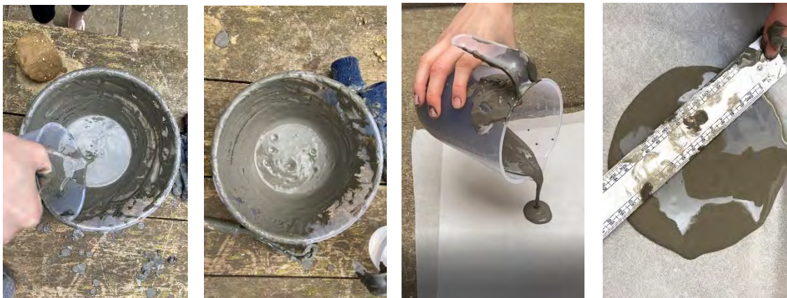
Figure 20. Slip puddle test for thermal cob mix. Photos: Olivia Elsey (2022).
