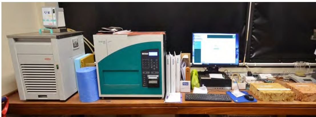
Figure 18. An example of a heat flow monitoring apparatus & thermal cob test sample. Photo: Plymouth University, CobBauge project.
