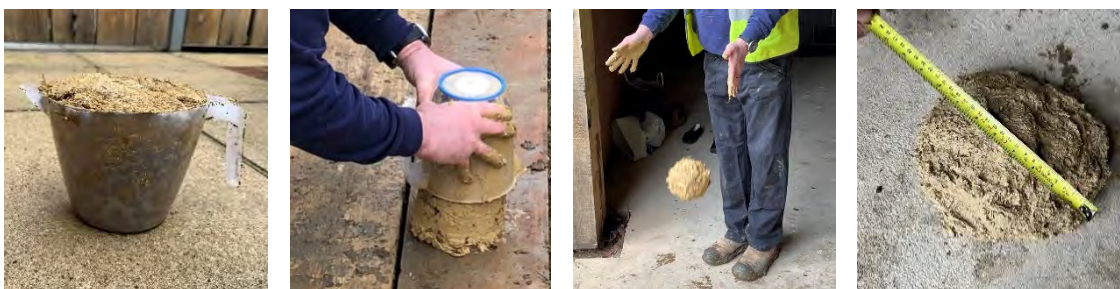
Figure 19. Ball drop test methodology for structural CobBauge mix. Photos: Katey Oven (2022).
