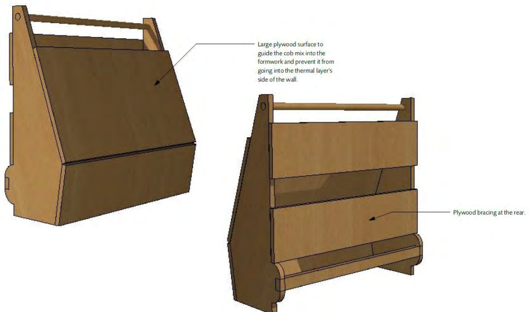
Figure 26. 3D views of CobBauge placement. Source: Hudson Architects (2022).
